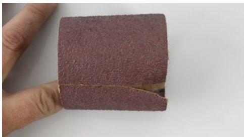
Step 1: Assure the direction of the seam on the sleeve is placed in this orientation on your arbor.
