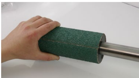
Step 4: Apply vacuum and slid the sleeve the rest of the way onto the arbor.
